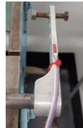
Figure 6 – Strain gauge testing on ARB lever
