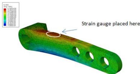
Figure 5 – Abaqus strain gauge testing
