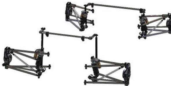
*Figure 4 - QFR '18 Pull rod suspension and Anti-roll system*
